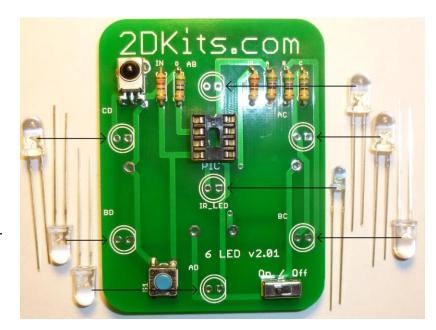
Now to solder in the battery clips and the pin back. Flip the board over, as these components will be inserted from the other side.
