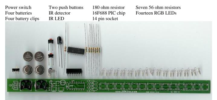
Got everything to start? If not, give us a shout. Also, since we pre-solder the battery clips, sometimes the switches or IR detector gets hidden under the battery clips.
