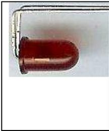
Make a 90 degree bend in the legs (leads) of the LED right at the surface of the LED. Make another 90 bend, so when inserted, the leads will fit in the board and the LED will fit in the hole.
