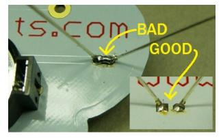
Take care to avoid a <u>bridge</u> of solder between the two leads of the LED. Current will flow through the bridge, and not the LED, thus the LED will not light up. This will also quickly drain the battery Fortunately, this is <u>easy to fix</u> – see details in the left column.
