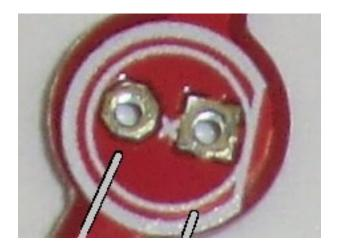
12. Turn the power switch off. Flip the board over and solder the LEDs. Keep the LED tight against the circuit board so it looks nice. That also means holding it down for a bit after removing the soldering iron, until the solder cools – just a few seconds.
