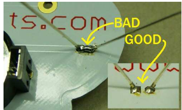
A bridge between the two leads of the LED. Electricity will flow through the bridge, and not the LED, thus the LED will not light up. Fortunately, this is easy to fix.
