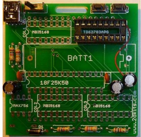
8. Insert the 16 pin single header sockets. **Be careful!** These must be inserted from the correct side. If you can see the silk screening for the headers, they are being inserted correctly. **Please re-check the placement again.** Flip the board over and solder. Flip the board over.
