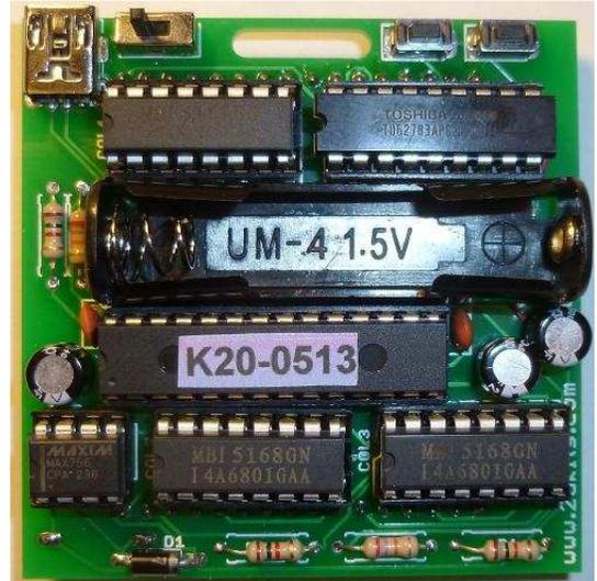
The AAA battery in conjunction with the MAX756 charge pump is not sufficient to drive all LEDs at once. Some patterns will look different when driven by just the AAA battery versus connected to the USB port. We have found a 3.7V battery in a AAA package does drive all LEDs as expected. We do have those available.
