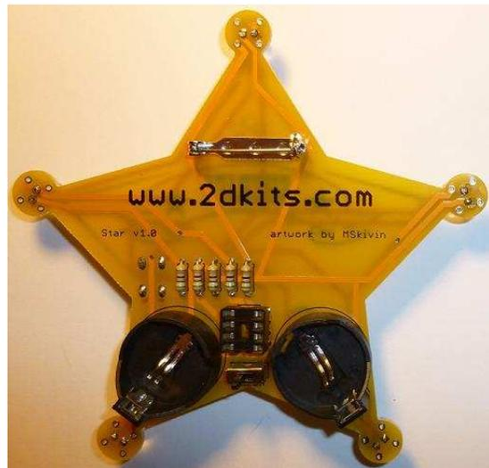
10. Flip the board over and insert the PIC into the eight pin socket. The small notch or dot on the PIC must down toward the bottom of the circuit board.
