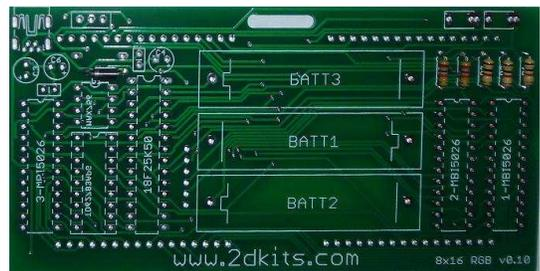
6. Insert the disk capacitors. They will be inserted on the upper left-hand portion of the circuit board. They can be inserted either way as orientation is not important for disk capacitors. Flip the board over and solder. Trim all the leads and flip the board over.
