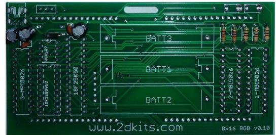
8. Insert the sockets. The notches on all the sockets must face to the top of the board. To keep the sockets from falling out when flipped, bend over two of the pins after each one has been inserted. Flip the board over and solder all pins. Trim the leads.
