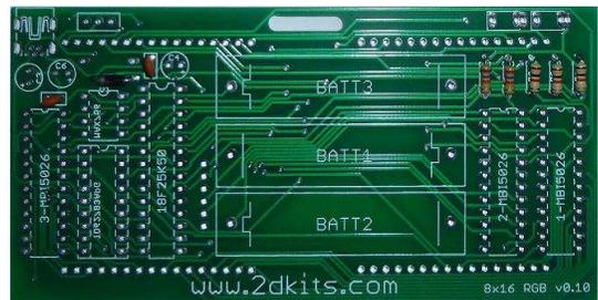
7. Insert the electrolytic capacitors at C3, C4, and C6. **Orientation is important** for electrolytic capacitors. Remember: **Short lead, square pad. Long lead, round pad.** Also, the positive (long lead) will match up with the “+” silk screen marking. Flip the board over and solder. Trim all the leads and flip the board over.
