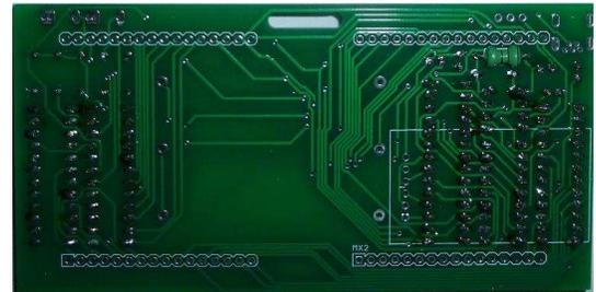
10. Insert the micro SD card module circuit board. Flip the board over and solder. Trim the leads.
