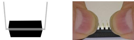
20. Flip the board back to the socket side, and insert the chips in the sockets. There are 4 chips, but only 3 different chips, each with a unique number of pins. Just match the chip size to the socket size. For each chip:
