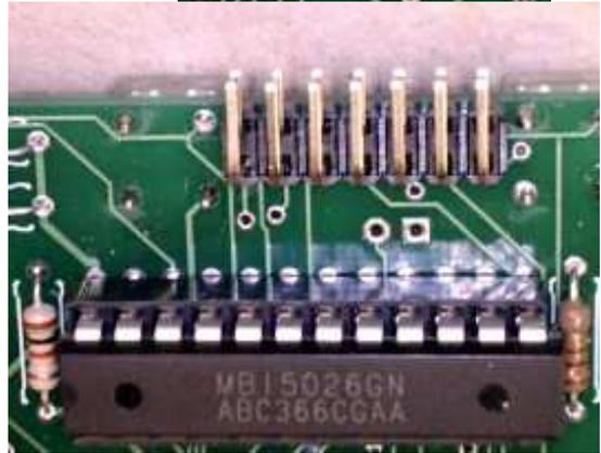
28. Caution: Overheating while soldering can cause the pins to slide – correct any such by re-melting the solder and sliding them back into position.
