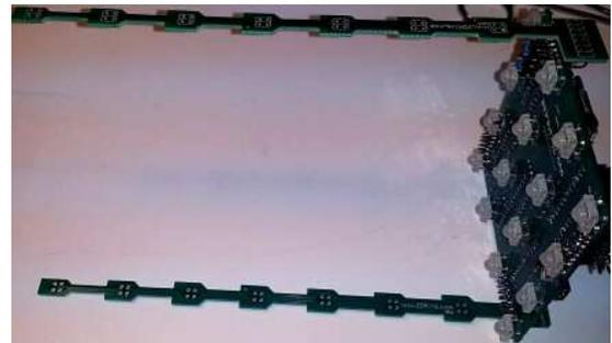
38. One by one, plug in the “waffle” boards being very careful to match “TOP” on waffle to “TOP” on base board, then top on the next waffle board to the other “TOPs”.
