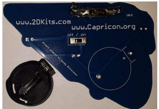
4. Flip the board over. Insert the battery. The plus sign “+” will face up. Angle it into the battery holder on the left side first, and then press down. It will snap in place. Verify the power switch is on. In the next few steps, the LEDs will be inserted and tested before they are soldered into the board.
