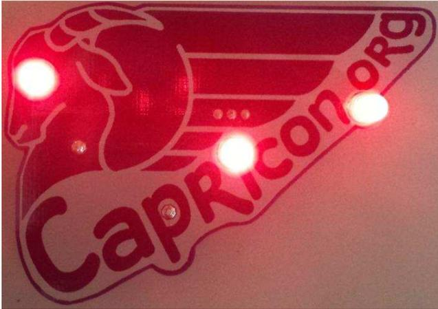
This blinkie is the Capricon Goat logo in a thin blue circuit board with three blinking LEDs.
