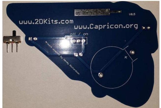
2. Flip the board over and solder the pinback. It will take a bit more time to heat up, so hold the soldering iron firmly against the base of the pinback and wait for the solder to flow.
