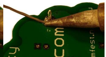
4) Remove the soldering iron
