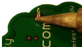
3) Keep heating to flow the solder
