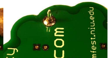
4) Remove the soldering iron
