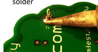
3) Keep heating to flow the solder
