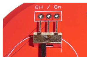
Insert switch into the holes inside the rectangular outline
