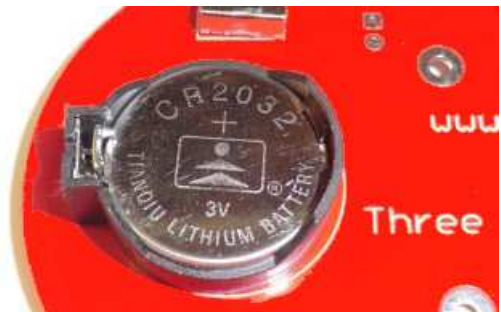
Close-up of soldered battery holder pin. Pad is covered with solder.
