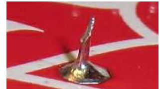
Close-up of soldered battery holder pin. Pad is covered with solder.
