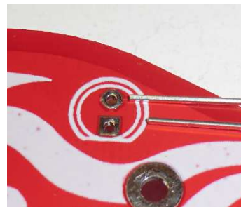
Inserting the LED: Long lead, round hole, short lead, square hole,
