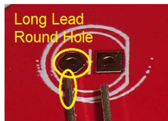
Insert long lead, round hole on the FRONT as shown.
