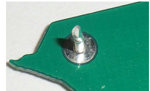
Flip to the Back to solder the pins
