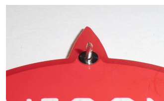
Flip to the Back to solder the pin
