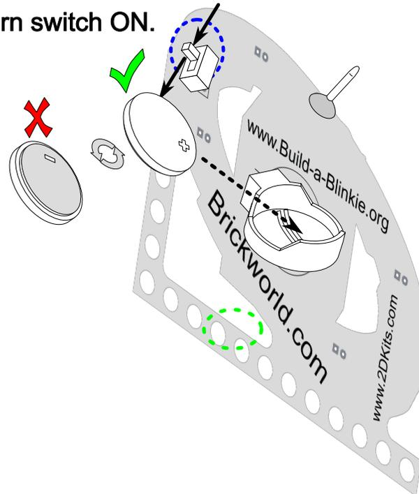
Insert battery, flat side up. Slide edge in, then push down to snap into place.
