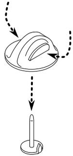
Remove tack from clasp by squeezing sides.
