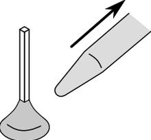
When solder flows across parts, remove iron. The solder will cool and harden in seconds.
