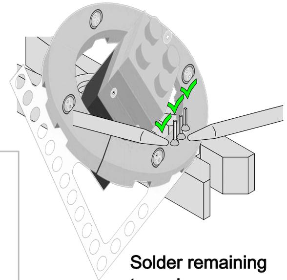
Solder remaining two wires.
