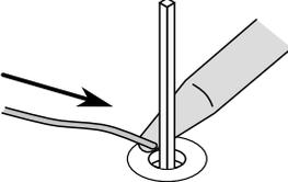
Melt about 1/2 inch of solder into joint.
