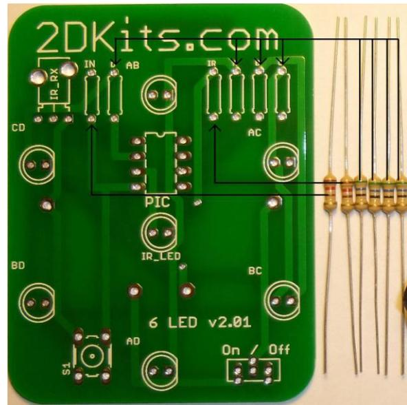
Solder in the IR detectors, 8 pin socket, push button, and power switch.
