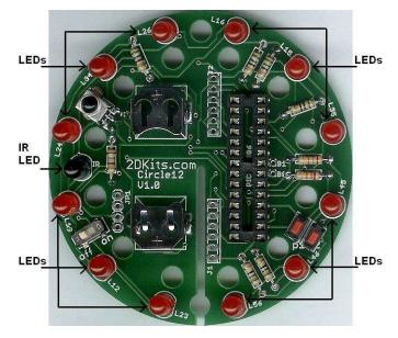
Insert the LEDs from the side as shown. Since both sides are silk screened (white printing), it is the side that has the L23, L12, L13, L24, L34, L26, L16, L15, L35, L45, L46, and L56 labels. Insert the LEDs at those locations. Then flip the board over and solder. **Orientation is important** for LEDs. Remember: **Short lead, square pad. Long lead, round pad.**
