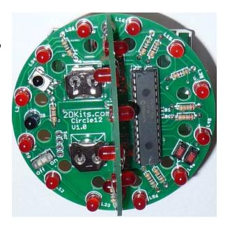
This kit contains two circuit boards – one with the battery clips, and one without. First, open up the kit and review the contents. Looking from left to right, and top to bottom there should be the following parts:
