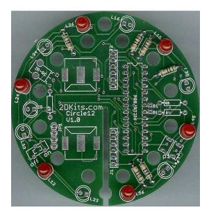
Note: Do not solder the bottom two LEDs (in the above picture), on either side of the slot, labeled L23 and L56. You will solder them in **after** the two boards are slid together!
