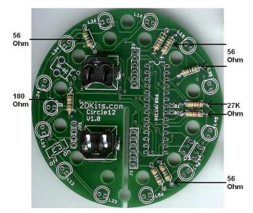
4. Once all the resistors have been soldered in, trim off the excess wire (leads).
