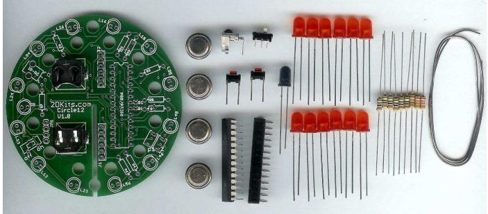
Circuit board Four LR44 batteries IR detector Power switch Two push buttons 16F886 PIC 28 pin socket IR LED Twelve LEDs Six 56 ohm resistors One 180 ohm resistor Two 27K ohm resistors Length of solder
