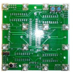
6. Flip the board over and insert the five sockets. Make sure the pin one indicator on each socket matches the correct position on the silk screening. Flip the board over and solder in the five sockets.
