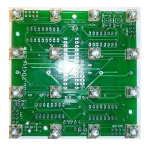
3. If your LED looks like this, you will need to reheat the solder joint while gently pressing down on the LED to make it sit level on the board. To this for any LEDs that are not level.
