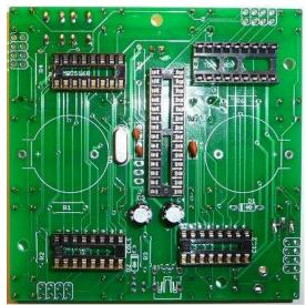
9. In the next few steps, diodes and resistors will be inserted. It is easier to insert them in you pre-bend the leads as shown.
