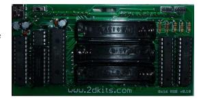
16. Insert the three AAA batteries. Alternatively, connect to a USB charger \*or\* to a USB cable connected to a USB port. Turn on the board and enjoy. The length of battery life depends on the number of LEDs lit at any one time. If the patterns are looking less colorful, replace the batteries, or plug into a USB port. Note, the USB does \*not\* recharge the batteries.
