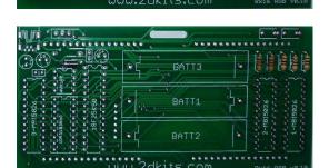
6. Insert the disk capacitors. They will be inserted on the upper left-hand portion of the circuit board. They can be inserted either way as orientation is not important for disk capacitors. Flip the board over and solder. Trim all the leads and flip the board over.
