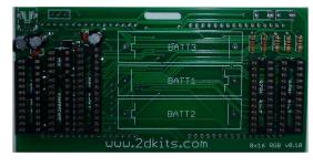
9. Insert the coil at L2. The coil can be inserted either way as orientation is not important for the coil. To make inserting easier, pre-bend the leads as was done to the resistors. Flip the board over and solder. Trim the leads.
