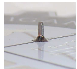
Close-up of soldered pin
