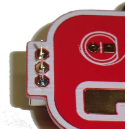
After soldering ONE pin
