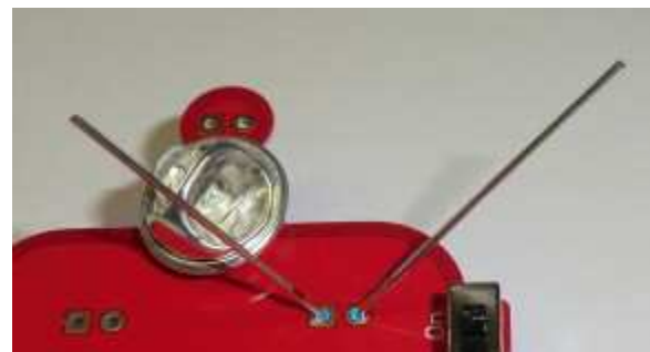
Bending the wires into a “V”
